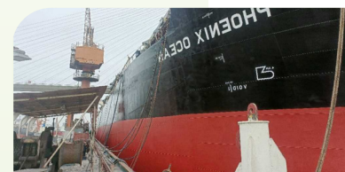
I Anticorrosive coating on PHOENIX OCEAN
