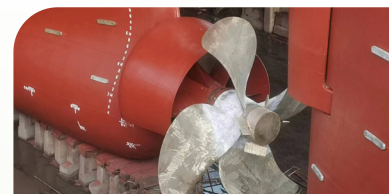
I Duct and propeller boss cap fins on EGRET OASIS
